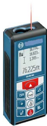
Figure 5-1: Laser-based equipment used to measure: (a) distances and (b) tilts (Bosch™)
